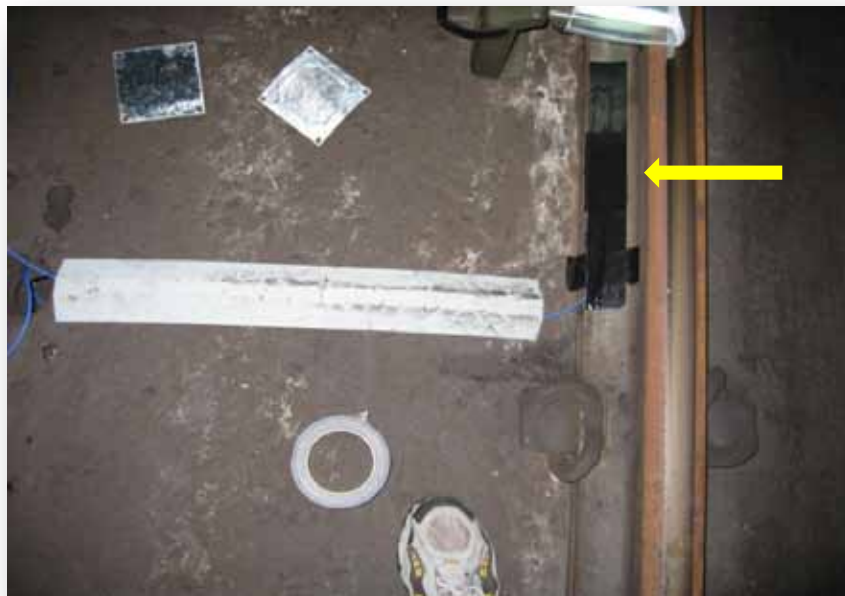
FBG strain sensor installed on the track.
