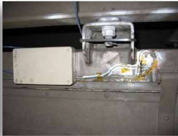
FBG Sensor on train charger, under carriage welding point.
