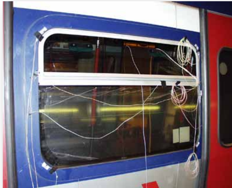
Strain gages instrumented on a train for assessing its structural integrity.
