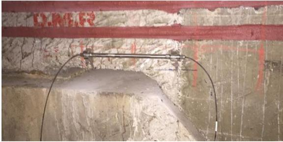
**Figure 5 os3610 Sensor Installed on Stepped Joint Nib**
