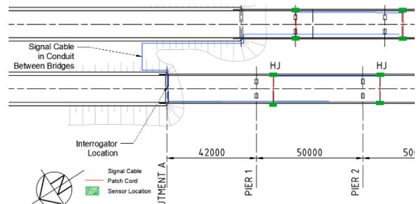
**Figure 7 Plan View of Monitoring System**
