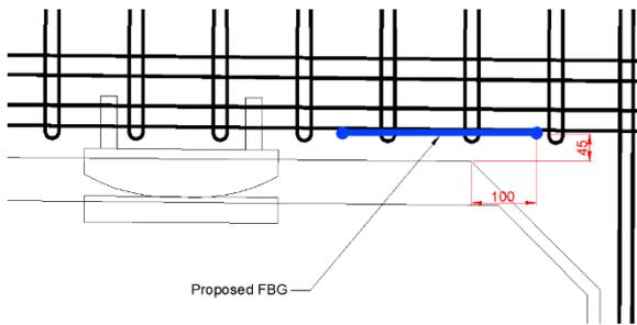
**Figure 3 Detailed Location of Strain Sensing Device**
