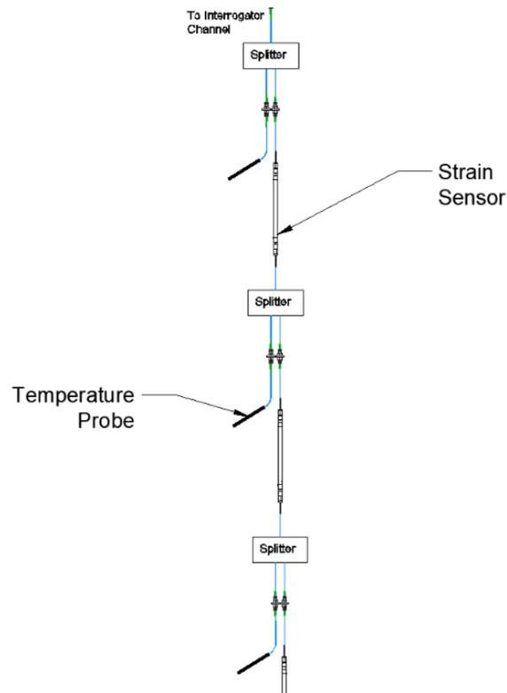
**Figure 8 Multiplexing the Temperature Probes**
