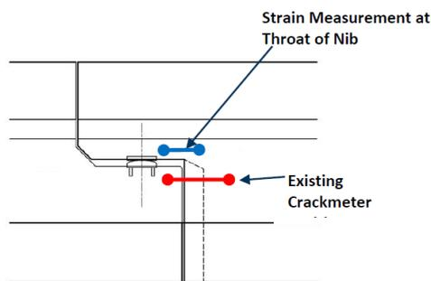
**Figure 2 Proposed Location of the Strain Sensing Device**
