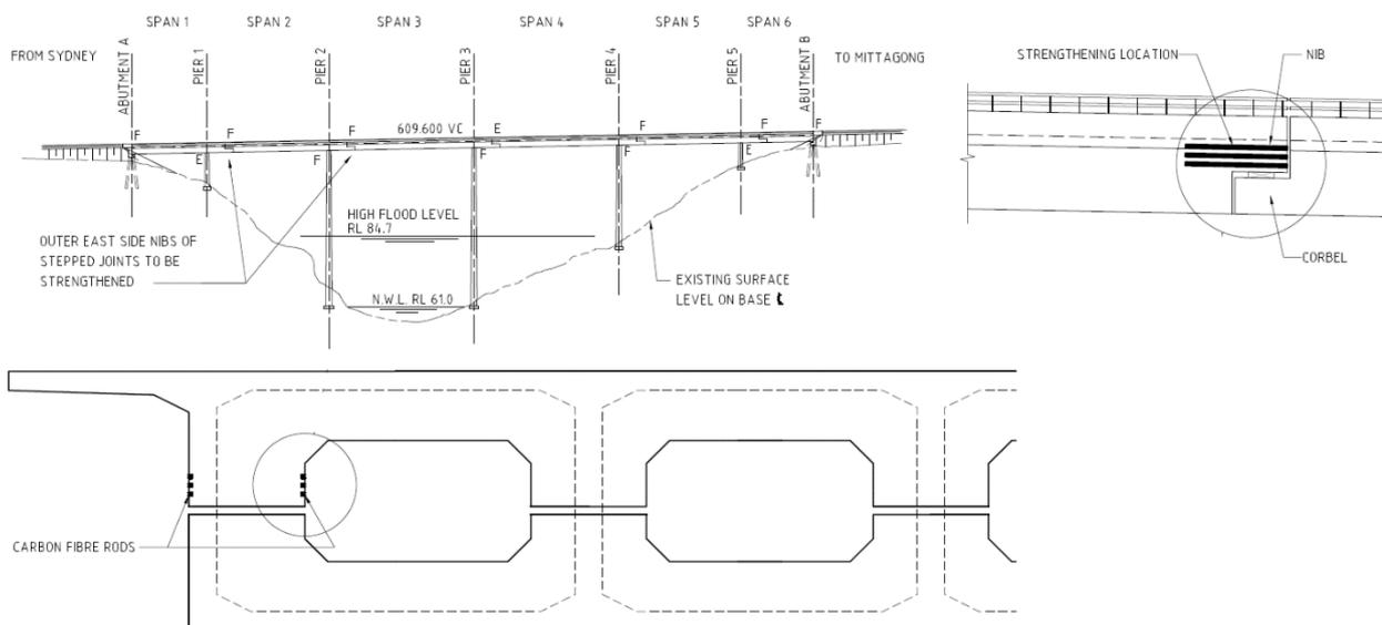
Figure 1 Reinforcement of Stepped Joints
