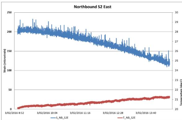
**Figure 13 Eastern Stepped Joint Trial Data in February 2016**
