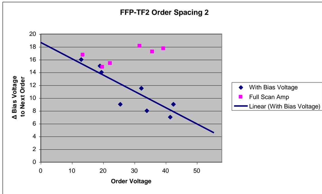
**Figure 2. Using limited 18 Volt scan amplitude, Volts/FSR parameter varies strongly as a function of bias voltage applied to PZT. Driver circuit design parameters can be modified to account for these behaviors.**
