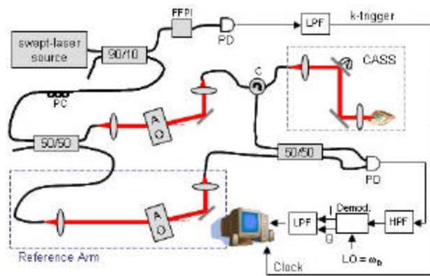
**Figure 1.** Heterodyne swept-source OCT system utilizing acousto-optic modulators. The swept-laser source has a center wavelength  $\lambda_0 = 1310\text{nm}$  and bandwidth  $\Delta\lambda = 100\text{nm}$ . A balanced detector is used for DC artifact suppression. FFPI: fiber Fabry-Perot interferometer; PC: polarization controllers; AO: acousto-optic modulator; C: circulator; CASS: anterior segment scanner.
