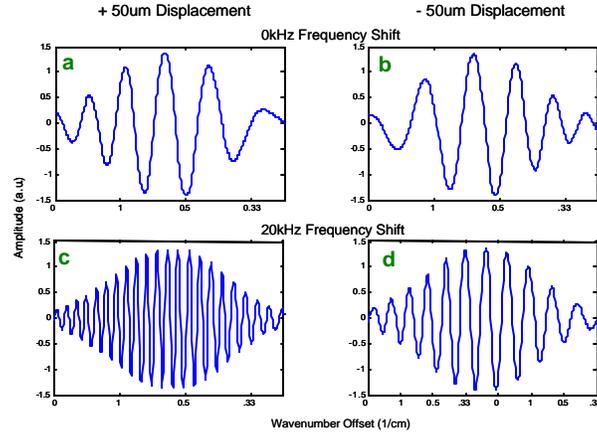
**Figure 2.** Interferograms taken using heterodyne SSOCT. (a) and (b) are taken from a reflector at +50 $\mu\text{m}$  and -50 $\mu\text{m}$  pathlength difference, respectively with a 0kHz frequency shift. (c) and (d) are collected at the same pathlength difference, but with a 20kHz frequency shift. By using heterodyne detection, reflectors at positive positions produce higher fringe frequencies than those at negative positions and therefore are unambiguously resolved.
