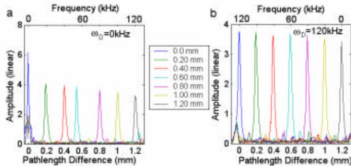
**Figure 3.** Falloff measurements for (a) homodyne and (b) heterodyne SSOCT. Heterodyne SSOCT enables frequency shifting of zero pathlength difference away from DC and auto-correlation artifacts, while falloff stays centered around zero pathlength difference. -50 dB reflector used in sample arm.
