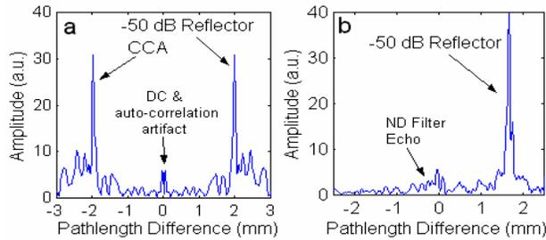
**Figure 4.** A-scans of a  $-50\text{dB}$  reflector at  $2.0\text{mm}$  pathlength difference. (a) A-scan showing unresolvable complex conjugate ambiguity (CCA) acquired using homodyne SSOCT. The CCA prevents distinguishing reflectors at  $+2.0\text{mm}$  from those at  $-2.0\text{mm}$  depth. Using heterodyne SSOCT (b), the CCA is resolved down to the noise floor of the system. The echo is a double-pass reflection from the ND filter, and shifts with the main reflector peak.
