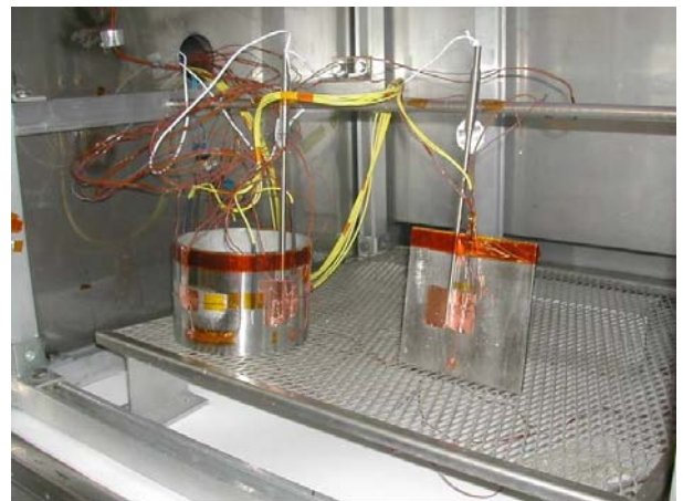
Figure 9. Fiber optic sensor for measuring temperature and heat flux (bench marking)
