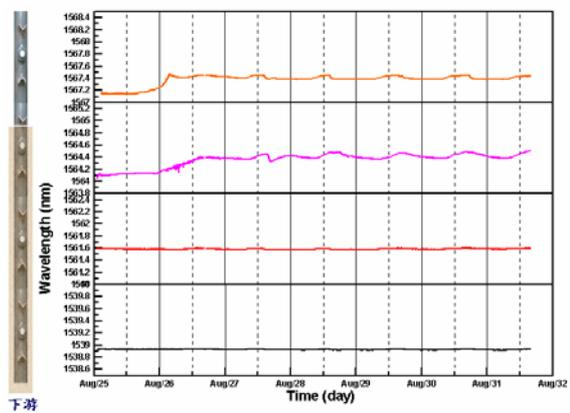
Figure 3 The measured data of the scouring processes from FBG sensors
