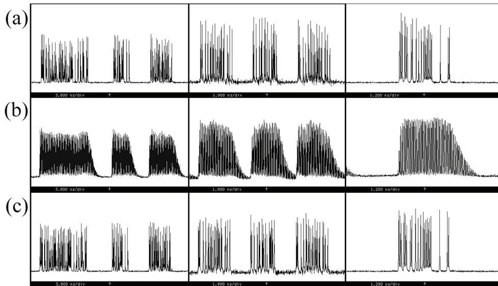
Fig. 2. Pulse traces. First column: synchronous operation (time scale 3.8 ns/div), second column: asynchronous operation (time scale 1.9 ns/div), third column: individual packet (time scale 1.2 ns/div). (a): input signal, (b): recovered clock, (c): recovered signal.
