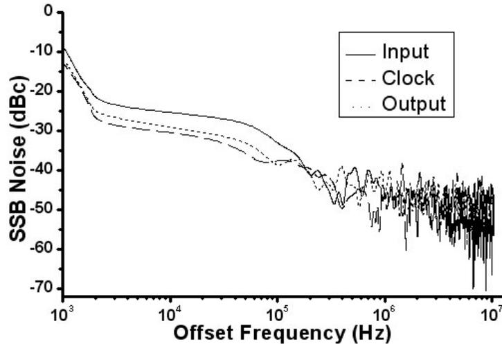
Fig. 4. SSB noise spectra of the input, clock and recovered signal.
