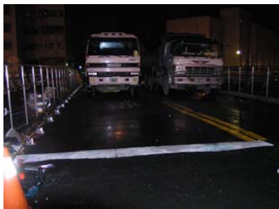
Fig. 6. Static loading test of the Ming-De Bridge
