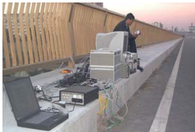
Fig.5. Measurement service on Hulanhe bridge (left), and FBG sensor display on Micron Optics FBG sensor interrogation system (right).
