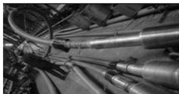
Figure 6 Smart cables based on FBGs
