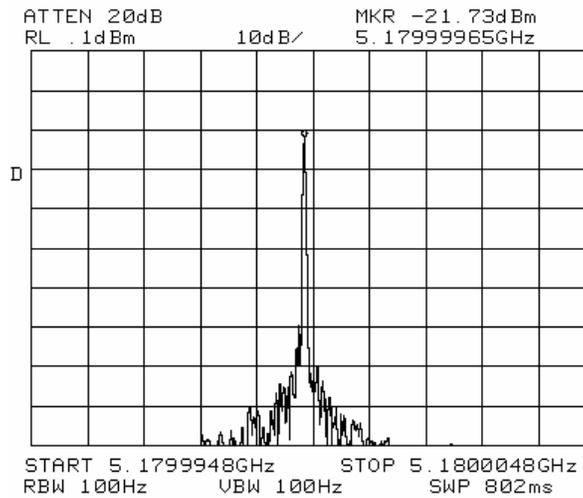
Fig. 3. RF spectrum around fundamental repetition frequency
