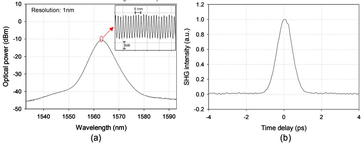
Fig. 2. (a) Output optical spectrum (b) SHG autocorrelation trace
