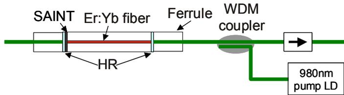
Fig. 1. Passively mode-locked FFPL with SAINT
