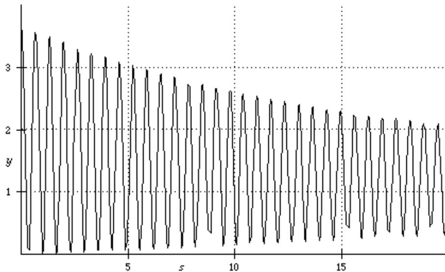
**Figure 4.2.-** EFFT light response signal as a function of fiber separation S
