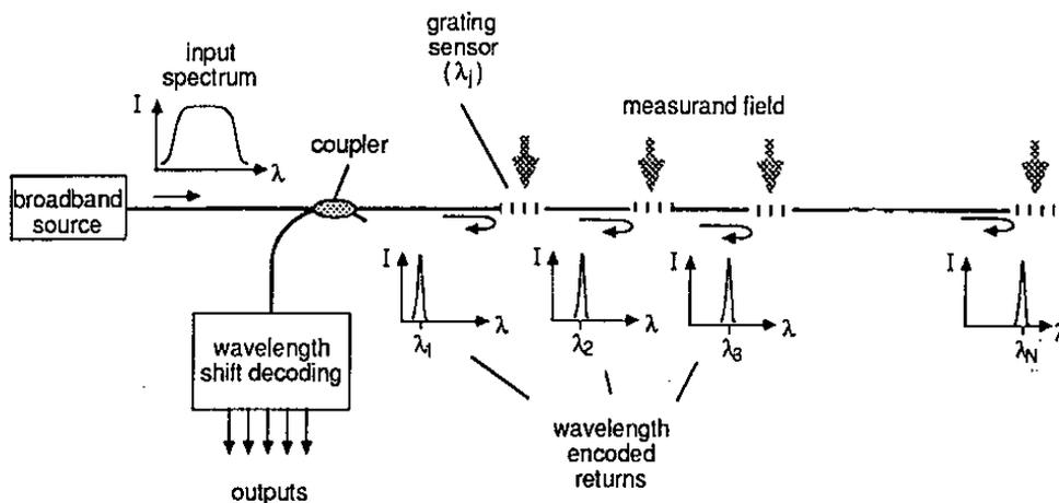
**Figure 3.4** Schematic representation of a WDM interrogation of a FBG array
