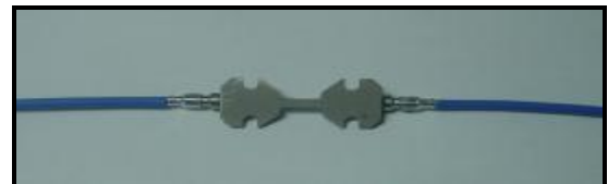
Figure 4. Sketch for mental slice encapsulation for FBG strain sensor
