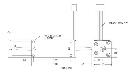
Figure 2 Mechanical dimensions of the all fiber phase shifter
