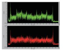
Figure 4. PM fiber coil manufacturing in-process monitoring. Green: In-line polarization x-talk measurement of a PM coil with quadrupole winding pattern from an initial winding trial. Red: In-line x-talk measurement of the same PM coil after adjusting winding procedure. The high x-talk peaks at cross-over points have been eliminated.
