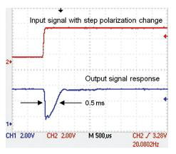
Figure 2 POS-002-I compensation for a step polarization change.
