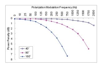
Figure 3. POS-002-I tracking of sinusoidal polarization modulation.
