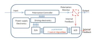
Figure 1. PolaStay™ polarization tracker function diagram. Either internal or external feedback can be used. Diagram shows structure for internal feedback.
