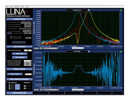
With a single scan, the OVA 5000 simultaneously measures the complete transfer function of photonic devices and subsystems. This screen shows IL and Group Delay versus wavelength.
