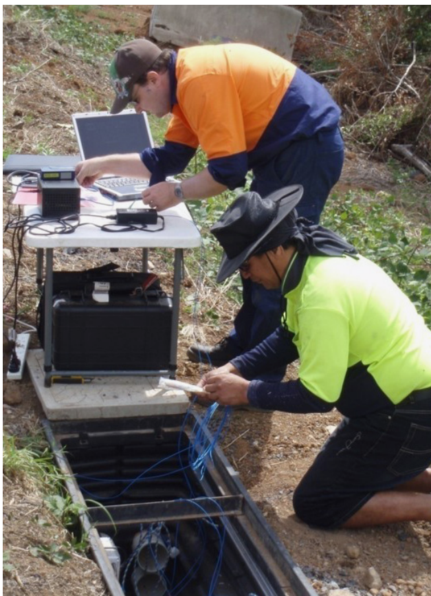
A Luna sm125 was used in the field for its proven reliability and accuracy
