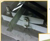
Displacement gages are mounted on the rocker bearings to monitor movement away from the supports as the bridge expands and contracts in response to changes of up to 70°C
