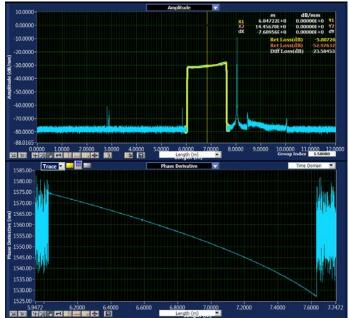
Figure 1: Phase Derivative (Wavelength) of Grating Versus Distance
