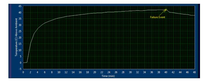
Figure 3. Time-lapse temperature plot of detector ADC 5. Again, system failure can be seen here after 40 minutes.
