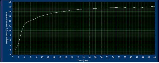
Figure 4. Time-lapse temperature of plot of laser ADC. The temperature continues to rise even after system failure occurs after 40 minutes.
