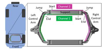
Figure 1. Instrumentation location underneath the vehicle. Two sensors were used to monitor the support beam and control arms on both sides of the vehicle. Channel 1 and 2 were instrumented in opposite directions on the support beam but identically on the control arms.
