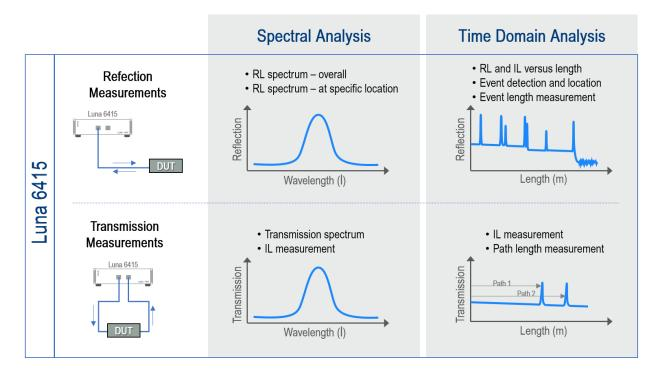
Figure 6. The Luna 6415 provides both traditional spectral analysis and time/length domain analysis of passive optical components; and is able to measure the loss of a DUT connected in reflection or in transmission
