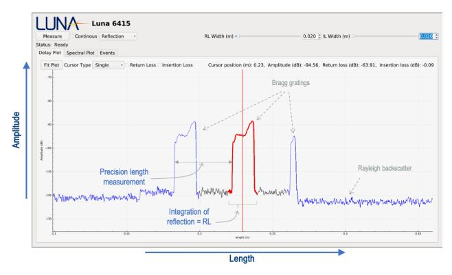
Figure 7. A scan of a Bragg gating string with a Luna 6415, connected in reflection, illustrates the high-resolution map of reflectance versus length, allowing high-precision measurement of RL, IL and path lengths
