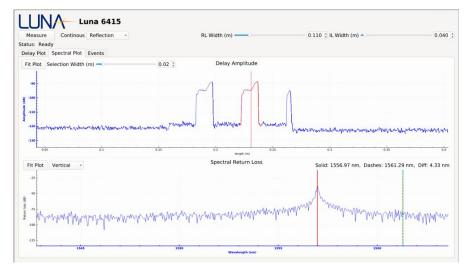
Figure 8. In the lower plot, the reflection spectrum of the second Bragg grating (selected and highlighted in red in the upper plot) is displayed
