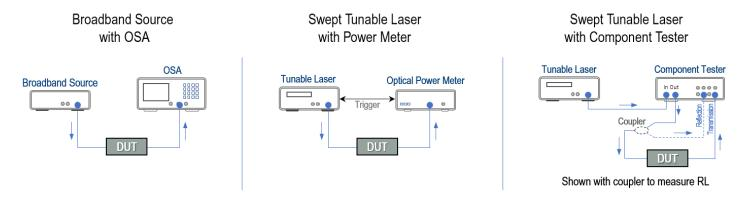
Figure 3. Traditional approaches to measuring component IL and RL with respect to wavelength
