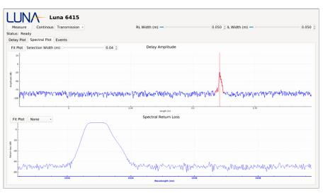
Figure 9. The transmission spectrum of an add-drop filter scanned by a Luna 6415 Lightwave Component Analyzer
