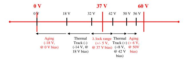
Figure 4. Modified Actuator Design Map with Design Parameter Corrections
