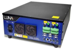
**How does it work?** The T-Ray 5000 Control Unit delivers precisely controlled optical signals to the T-Gauge Sensor Heads enabling them to generate and receive terahertz signals. The processed waveforms enable multiple measurements to be made simultaneously with a single sensor head.
