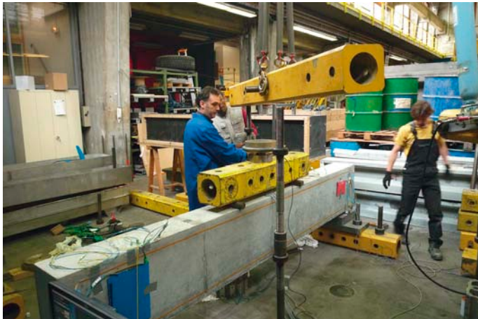
Figure 5: Load bearing test on a reinforced concrete girder that has an integrated fibre-optic cable which measures the strain using Rayleigh scattering (image source: [1])
