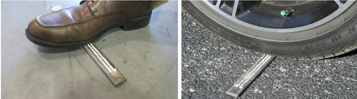
Figure 4: Fiber sensor with protective coating applied, being stepped on and driven across, with no degradation of data quality.
