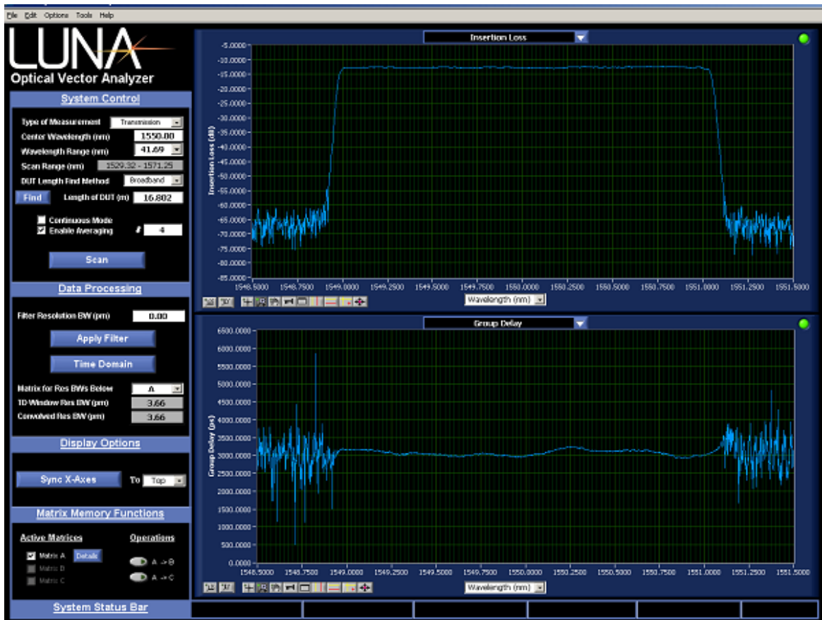
Figure 14. Insertion Loss and Group Delay of DCM with Compression Enabled
